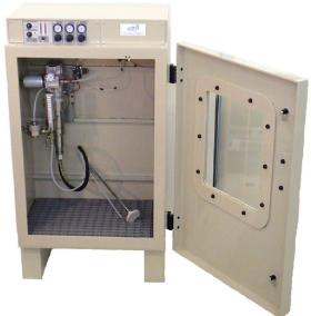
Automatic electrostatic system for water based paints, with insulation and medium pressure feeding. Can be used with high viscosity fluids, with stainless steel tank (optional). Stainless Steel Pump lower and fluid passages suitable for water base paints. Innovative electrostatic system with product, air, and voltage adjustments outside the cabinet. Automatic cleaning system, (optional).
